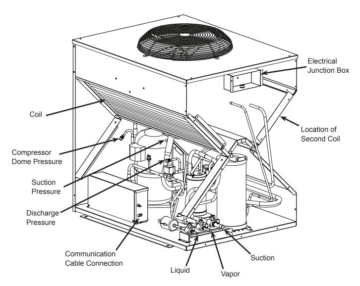
The electrical power supply connects to the wires in the junction box near the top of the condensing unit. The communication cable that connects to the ice making head routes thru a bushing near the base and routes to a connector on the side of the control box.
